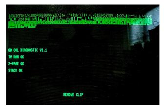
Now, those diagnostic boxes and clips are very rare – but it is now much easier to use a custom EPROM in the F000 socket, programmed with the Diagnostic ROM code and the original F000 ROM code and switch back to the original ROM when it says "REMOVE CLIP". This is also far more reliable than removing the test clip as supplied by Commodore, which would often crash the system under test.
