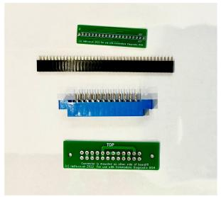
**DO NOT** pull on the PCB unless the connector is bolted to the board or you may damage the board as the edge connectors are initially quite a tight fit. Push the connector from INSIDE the PET case if required to avoid damaging the PCB until it loosens off a little.
